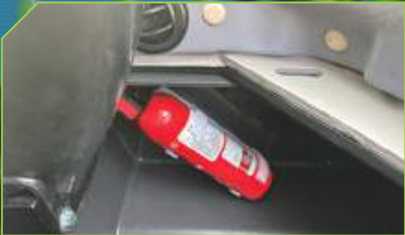
Optional fire extinguisher Designed layout, does not occupy the operating space, convenient and easy to contact, prevent emergency, protect the driver.
