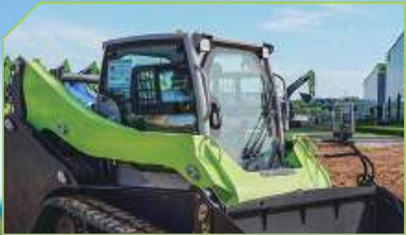
FOPS/ROPS cab A cab certified for FOPS/ROPS provides protection in the event of unforeseen rollovers and falling objects.
