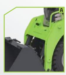
• Bucket cylinders and pipelines are equipped with protective cover to prevent from being damaged.
